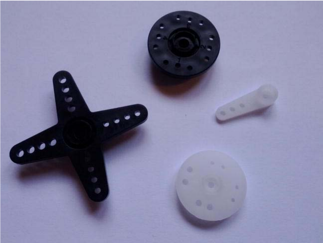
Figure 9-6. Servo drive shaft attachments
