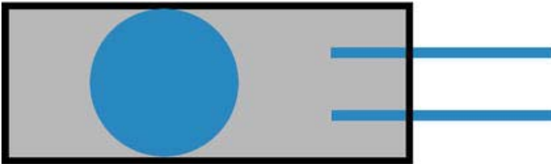
Figure 10-2. Open tilt-switch (inside view)
