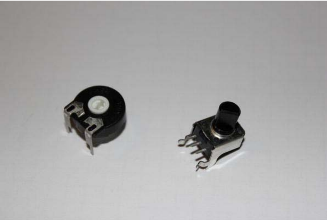
Figure 4-12. Potentiometer: trimmer (left), rotary potentiometer (right)
