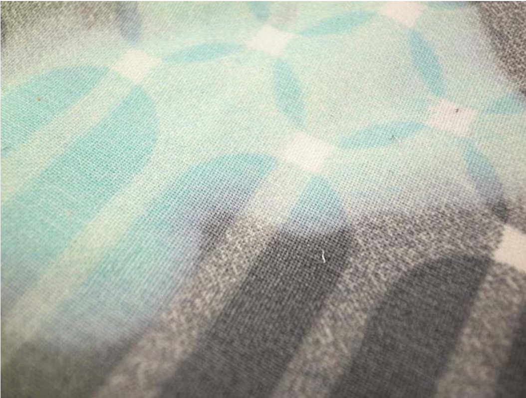
Figure 4-2. Thermochromic screen print after heat is applied
