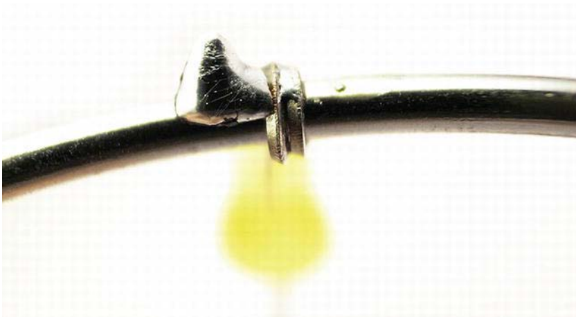
Figure 5-23. A cold soldering joint
