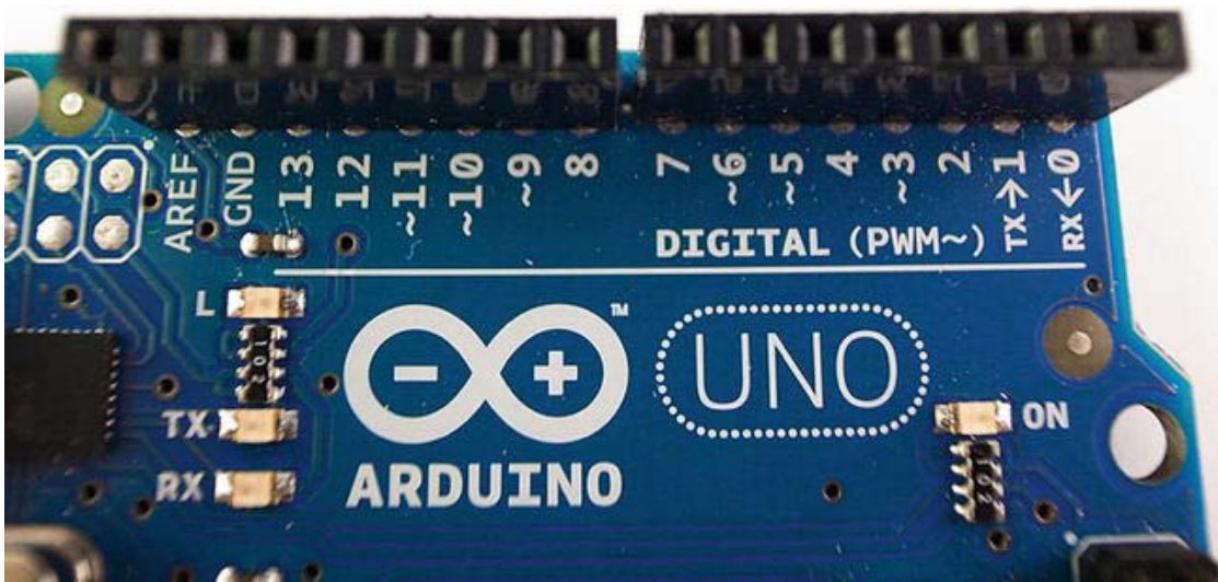
Figure 3-9. Digital pins from 0 to 13
