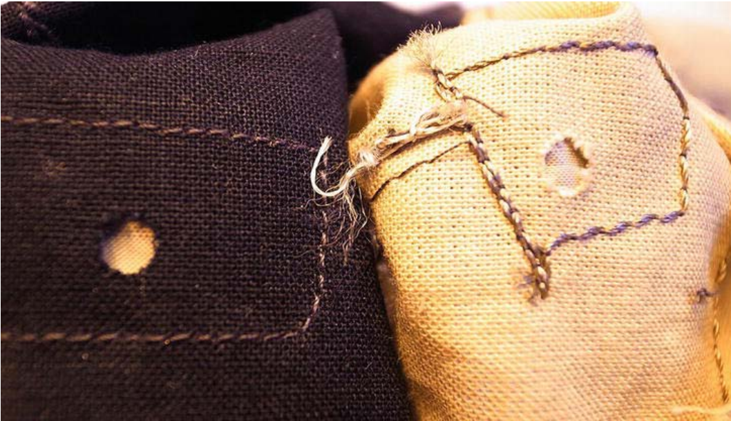
Figure 7-7. Conductive thread connections
