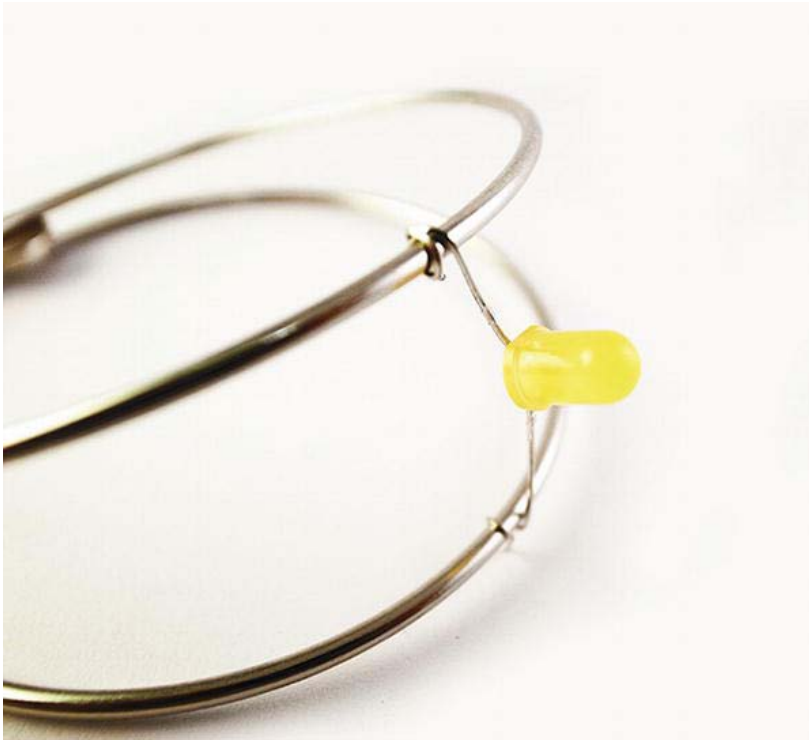
Figure 5-20. Wrapping the LED legs around the rings
