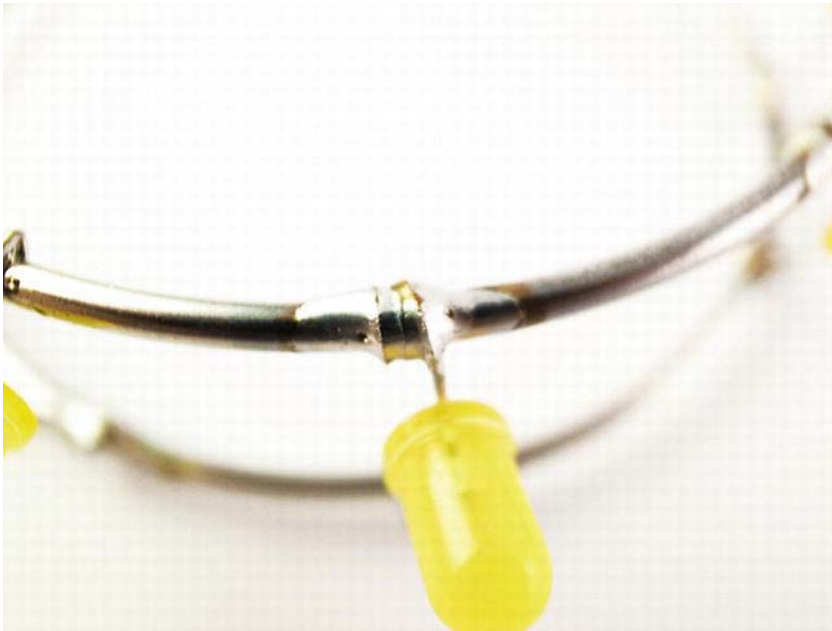
Figure 5-24. The solder should spread onto the material.
