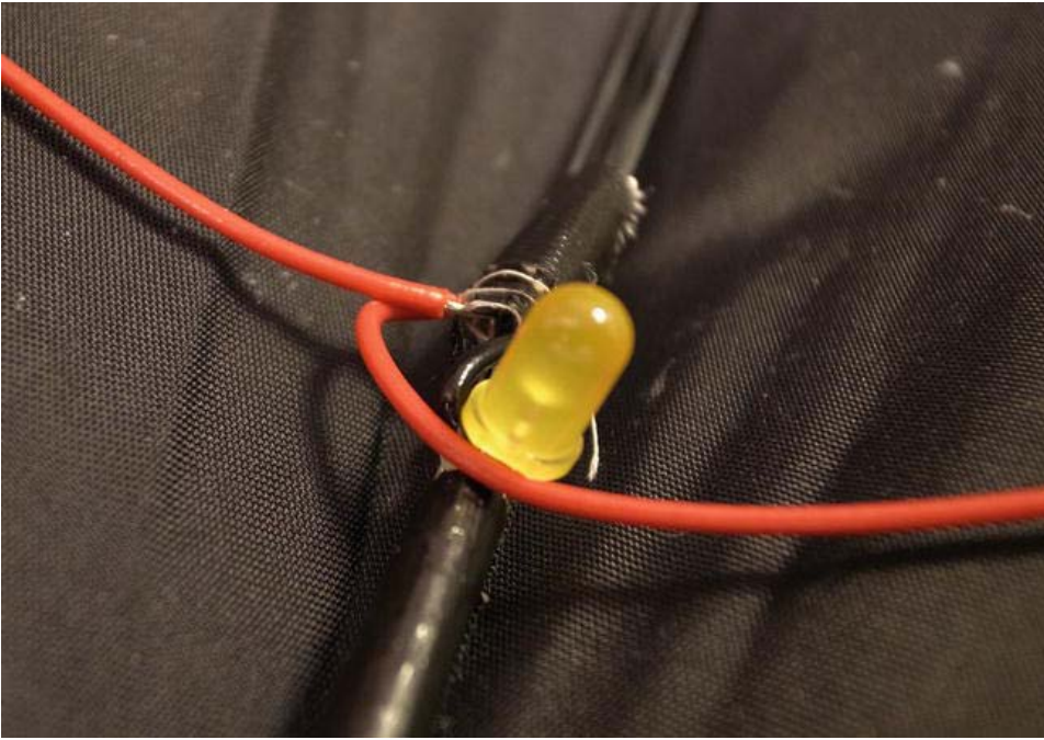
Figure 10-12. Adding the power wires around the umbrella
