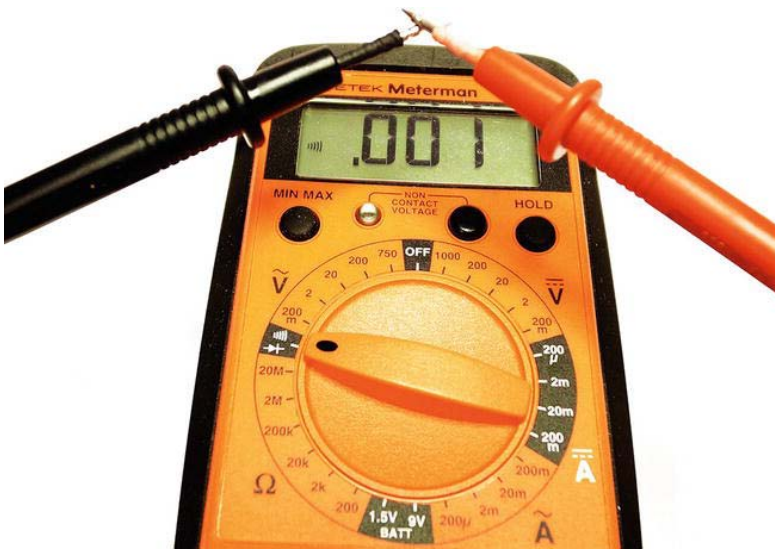
Figure 5-1. Finding conductivity with a multimeter
