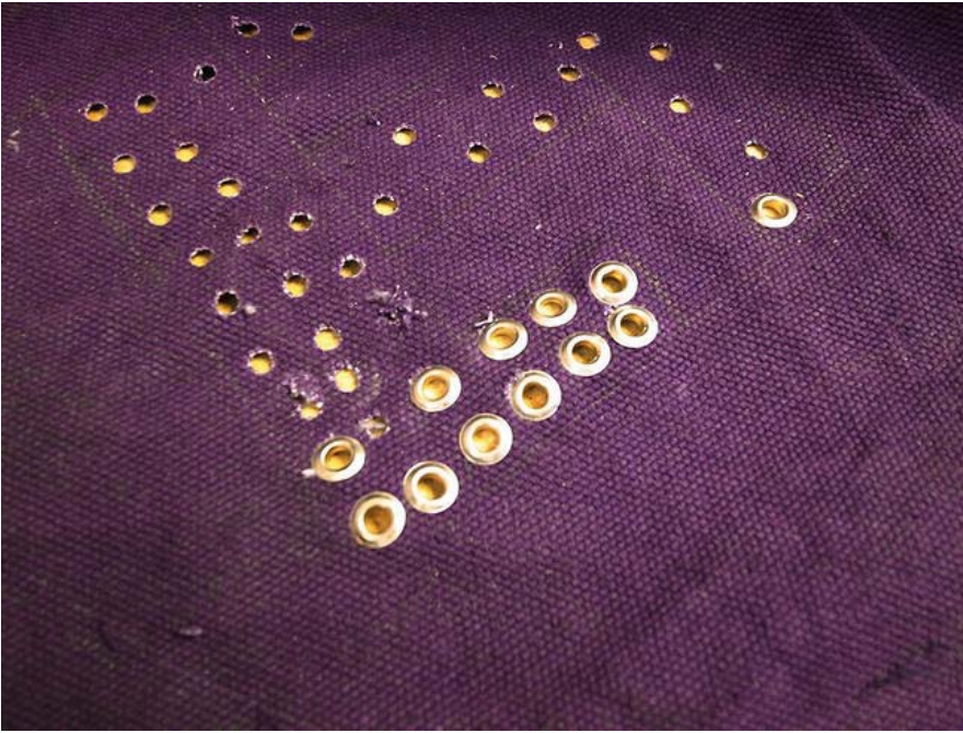
Figure 6-12. Eyelets punched in place
