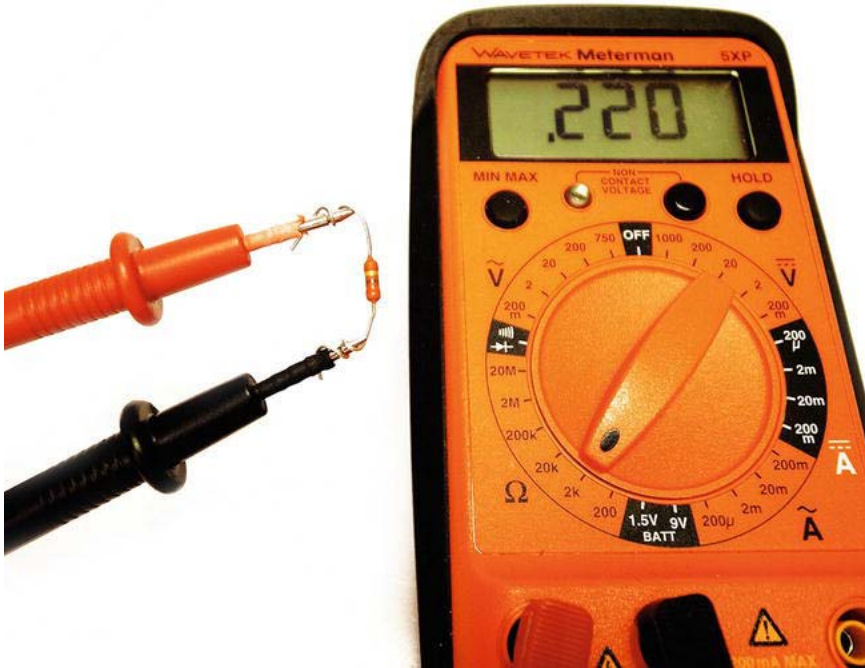
Figure 5-3. Measuring the resistance of a resistor
