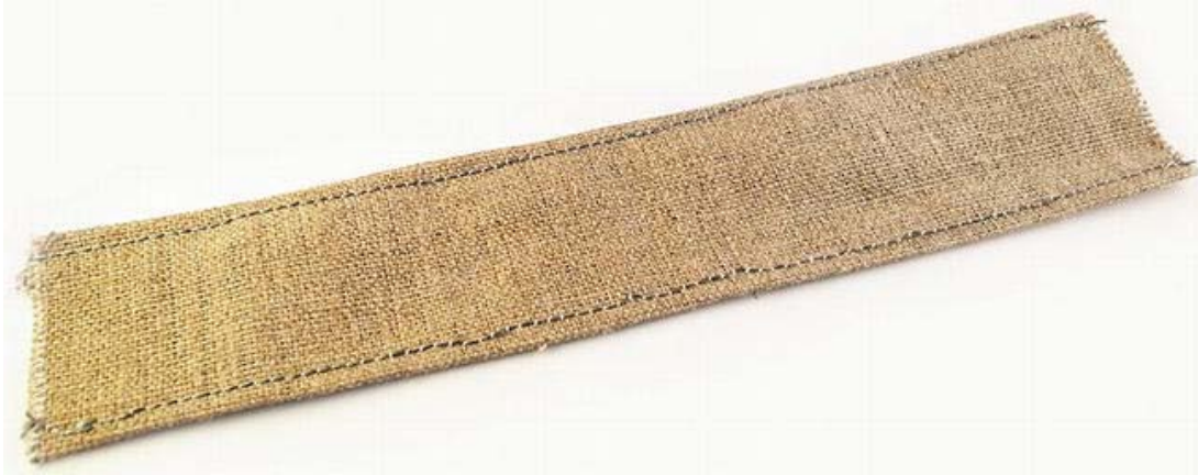
Figure 5-12. Seams sewn with conductive thread
