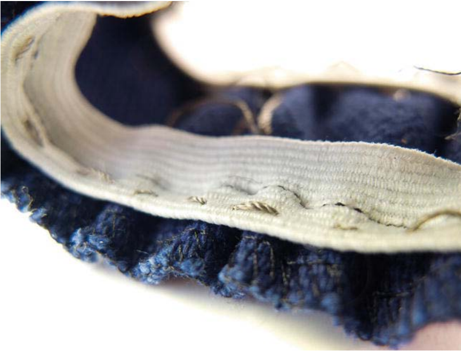
Figure 14-13. The extended ground connection between the battery and the ATtiny made with conductive thread into the elastic that connects to the skin
