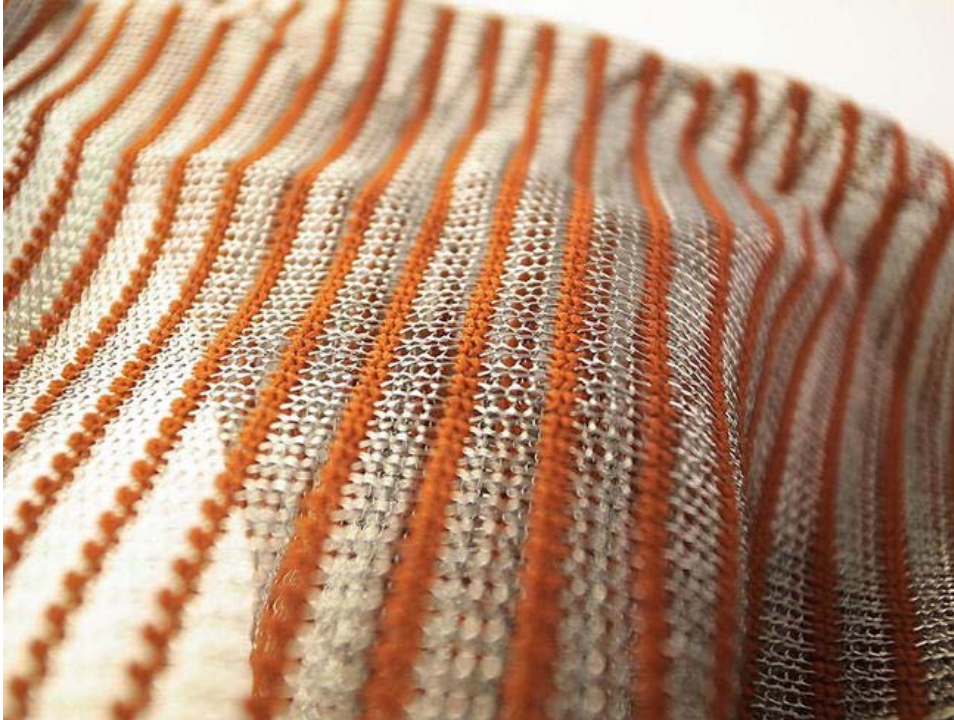
Figure 4-6. Conductive mesh fabric mixed with non-conductive thread
