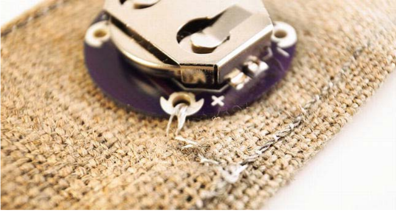
Figure 5-16. Making the power connection
