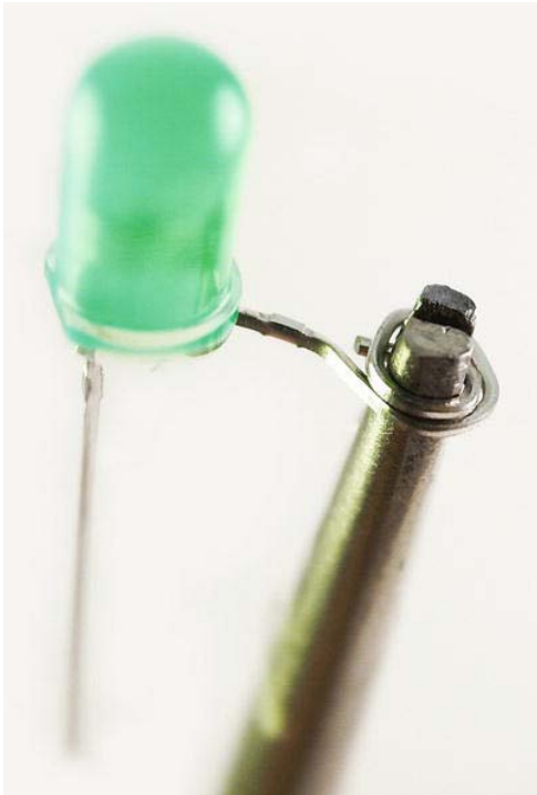
Figure 5-13. Modifying the LED legs
