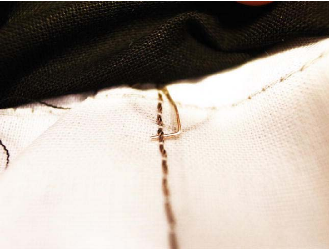
Figure 11-12. Hooking the LED to the conductive thread
