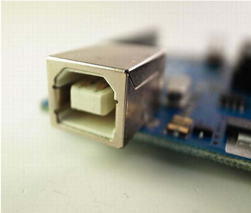
Figure 3-7. Close-up of the USB connector on a standard Arduino board
