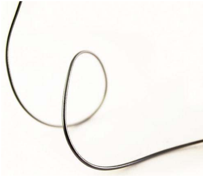
Figure 4-9. Smart wire that remembers shapes
