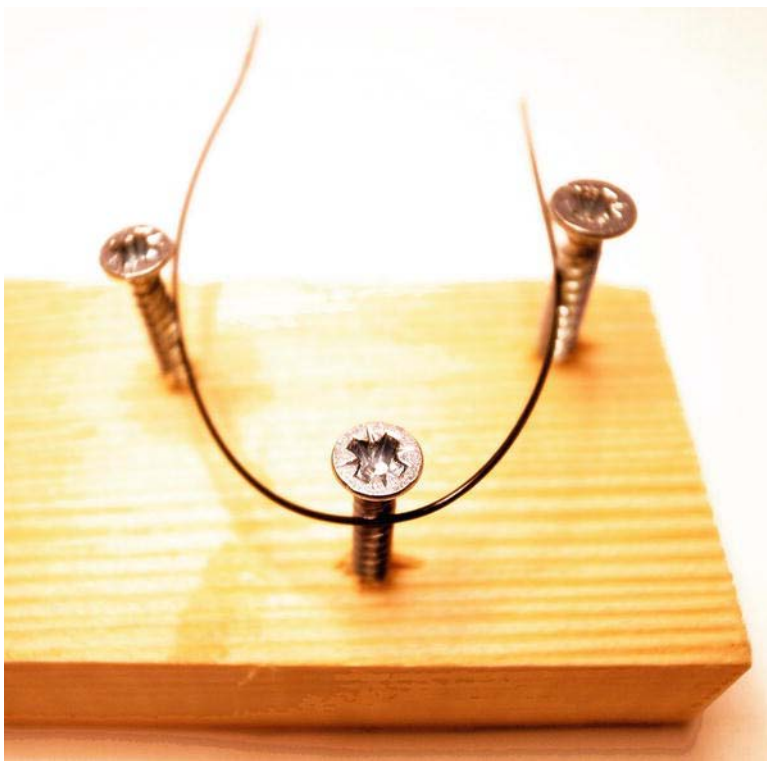
Figure 12-12. Reprogramming the SMA wire
